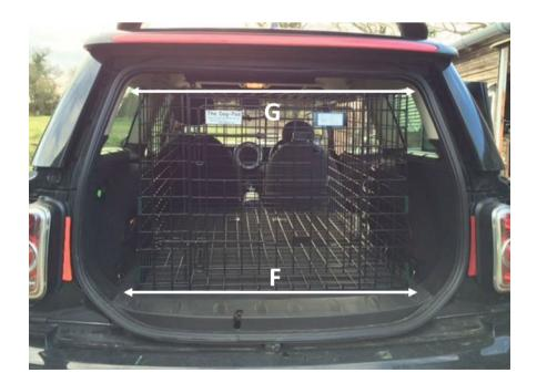
${\bf F}$  – width of the cage floor, this is governed by the space between wheel arches and the size of the rear door, accounting for any shaping at the corners
